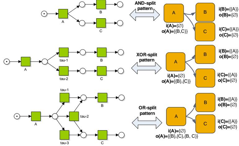
**Fig. 3.** Petri nets with invisible transitions labeled  $\tau$  (left) and their possible flexible model counterparts (right)
