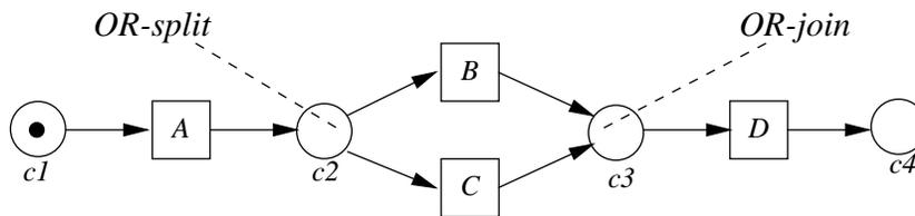
Figure 10: Conditional routing.
