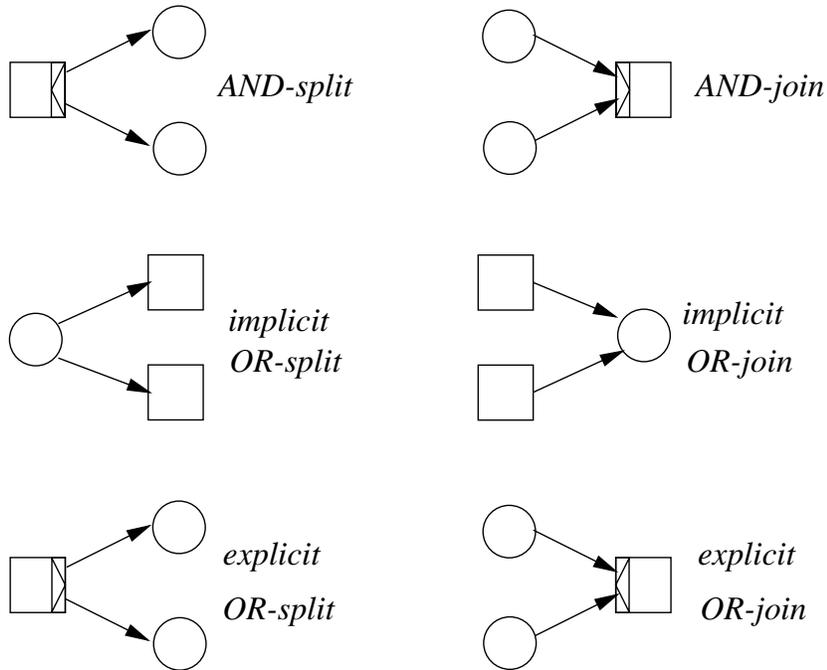
Figure 12: The building blocks for workflow modeling.
