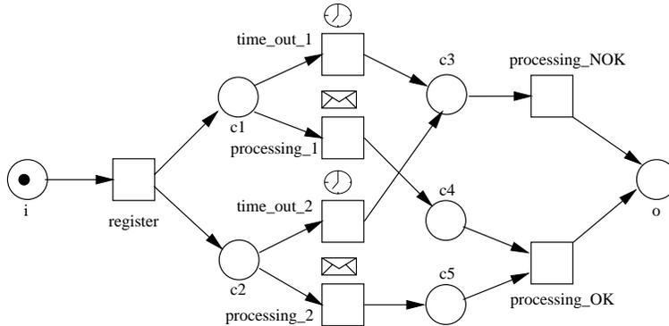
Figure 20: Another WF-net for the processing of complaints.
