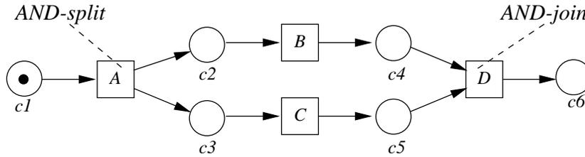
Figure 9: Parallel routing.
