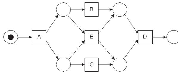
**Fig. 2.** A process model based on the event log shown in Table 1 discovered by the  $\alpha$ -algorithm.
