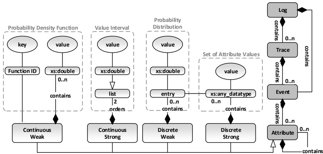
**Figure 1:** UML diagram illustrating an extension of the XES standard capable of representing uncertain data.
