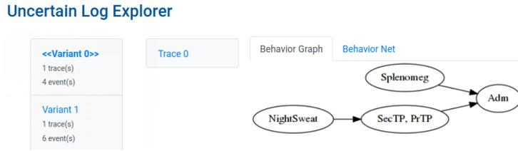
**Fig. 4:** The uncertain variant page of the PROVED tool, showing information regarding the variant obtained from the trace in Table 1. For a variant in an uncertain log, this page lists the traces belonging to that variant, and displays the graphical representations for that variant – behavior graph and behavior net (the latter is not displayed, but can be accessed through the tab on the top).
