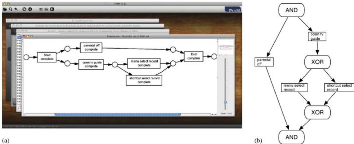
Figure 9. Discovered process model (a) in ProM and (b) conceptual visualization
