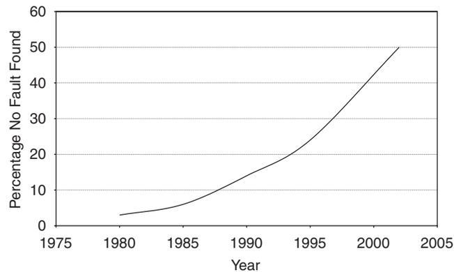
Figure 1. Rapid growth of 'no fault found' cases, where returned products seem to function correctly, in modern high-volume consumer electronics<sup>1</sup>
